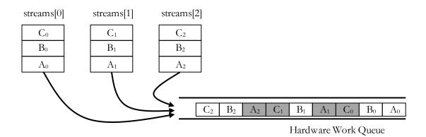
As a result the hardware is only able to determine that it can execute the shaded pairs concurrently.
