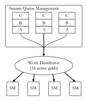
Using CUDA streams, we have declared the dependency chains  $A_0$ - $B_0$ - $C_0$  and  $A_1$ - $B_1$ - $C_1$  and  $A_2$ - $B_2$ - $C_2$ . Each of these chains is independent and therefore they could be executed at the same time (i.e. concurrently). With Fermi's single pipeline, however, this depth-first launch sequence will result in false dependencies:
