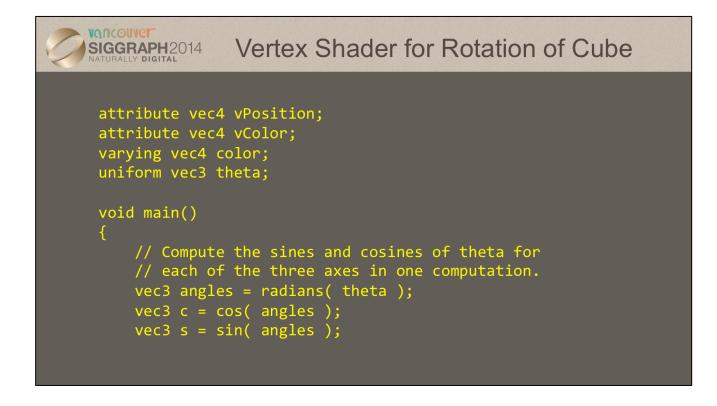
Here's an example vertex shader for rotating our cube. We generate the matrices in the shader (as compared to in the application), based on the input angle theta. It's useful to note that we can vectorize numerous computations. For example, we can generate a vectors of sines and cosines for the input angle, which we'll use in further computations.
