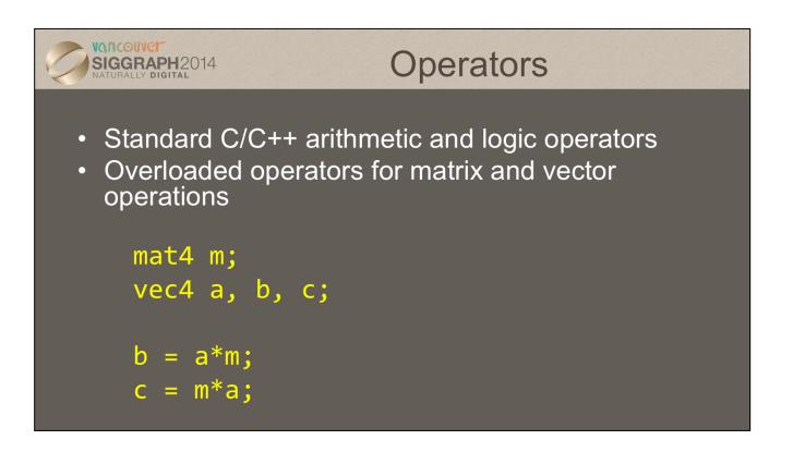
The vector and matrix classes of GLSL are first-class types, with arithmetic and logical operations well defined. This helps simplify your code, and prevent errors.
