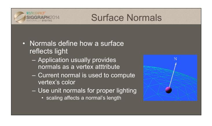
The lighting normal tells OpenGL how the object reflects light around a vertex. If you imagine that there is a small mirror at the vertex, the lighting normal describes how the mirror is oriented, and consequently how light is reflected.
