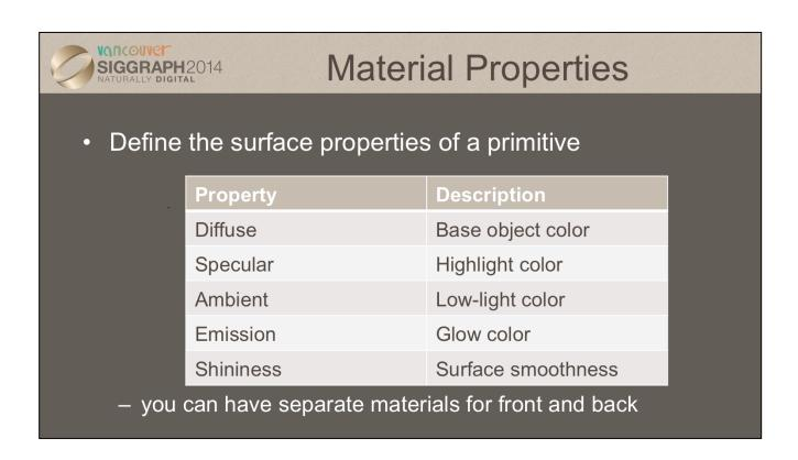
Material properties describe the color and surface properties of a material (dull, shiny, etc). The properties described above are components of the Phong lighting model, a simple model that yields reasonable results with little computation. Each of the material components would be passed into a vertex shader, for example, to be used in the lighting computation along with the vertex's position and lighting normal.
