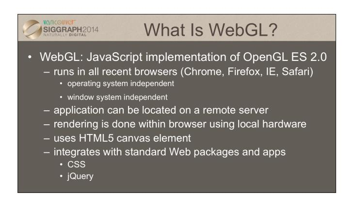
OpenGL ES is a smaller version of OpenGL that was designed for embedded systems which did have the hardware capability to run desktop OpenGL. OpenGL ES 2.0 is based on desktop OpenGL 3.1 and thus is shader based. Each application must provide both a vertex shader and a fragment shader. Functions from the fixed function pipeline that were in ES 1.0 have been deprecated. OpenGL ES has become the standard API for developing 3D cell phone applications.
