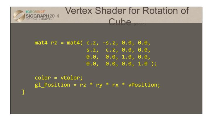
We complete our shader here by generating the last rotation matrix, and ) and then use the composition of those matrices to transform the input vertex position. We also *pass-thru* the color values by assigning the input color to an output variable.
