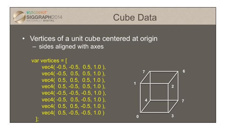
In our example we'll copy the coordinates of our cube model into a VBO for WebGLto use. Here we set up an array of eight coordinates for the corners of a unit cube centered at the origin.
