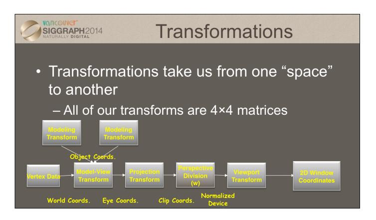
The processing required for converting a vertex from 3D or 4D space into a 2D window coordinate is done by the transform stage of the graphics pipeline. The operations in that stage are illustrated above. The purple boxes represent a matrix multiplication operation. In graphics, all of our matrices are 4×4 matrices (they're homogenous, hence the reason for homogenous coordinates).
