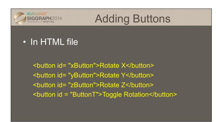
id allows us to refer to button in JS file. Text between <button> and </button> tags is placed on button. Clicking on button generates an event which we will handle with a listener in JS file.
