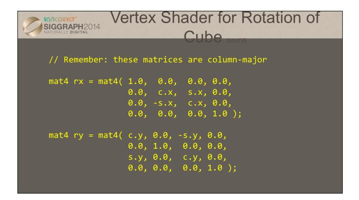
Completing our shader, we compose two of three rotation matrices (one around each axis). In generating our matrices, we use one of the many matrix constructor functions (in this case, specifying the 16 individual elements). It's important to note in this case, that our matrices are columnmajor, so we need to take care in the placement of the values in the constructor.
