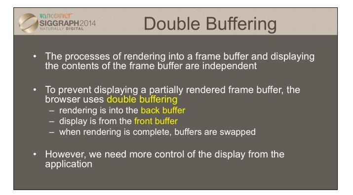
Double buffering is no faster or slower than single buffering. It just prevents the display of a partially rendered scene.
