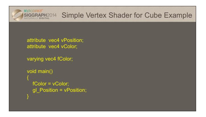
Here's the simple vertex shader we use in our cube rendering example. It accepts two vertex attributes as input: the vertex's position and color, and does very little processing on them; in fact, it merely copies the input into some output variables (with gl\_Position being implicitly declared). The results of each vertex shader execution are passed further down the OpenGL pipeline, and ultimately end their processing in the fragment shader.
