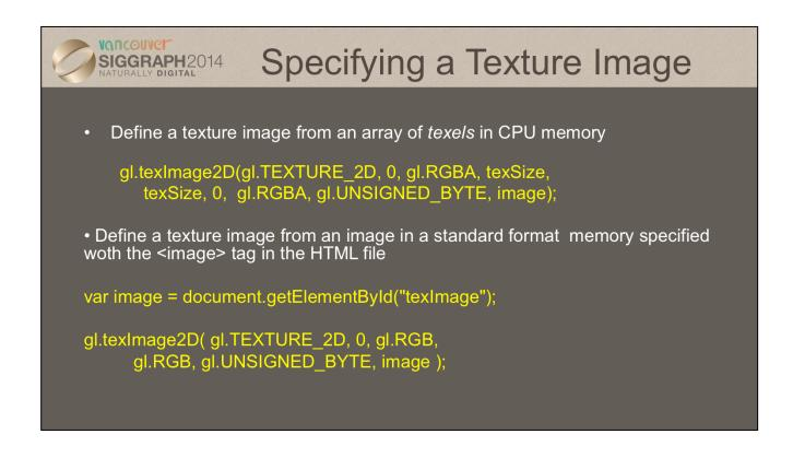
Specifying the texels for a texture is done using the  $gl.texImage_2D()$  call. This will transfer the texels in CPU memory to OpenGL, where they will be processed and converted into an internal format.
