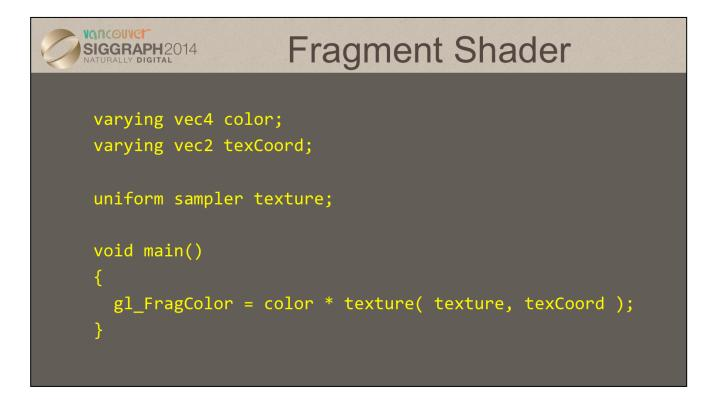
Continuing to update our shaders, we add some simple code to modify our fragment shader to include sampling a texture. How the texture is sampled (e.g., coordinate wrap modes, texel filtering, etc.) is configured in the application using the gl.texParameter\*() call.
