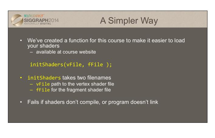
To simplify our lives, we created a routine that simplifies loading, compiling, and linking shaders: InitShaders(). It implements the shader compilation and linking process shown on the previous slide. It also does full error checking, and will terminate your program if there's an error at some stage in the process (production applications might choose a less terminal solution to the problem, but it's useful in the classroom).
