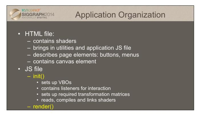
For a static application we can generate geometry in init() or call another function for init()
