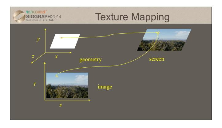
Textures are images that can be thought of as continuous and be one, two, three, or four dimensional. By convention, the coordinates of the image are *s*, *t*, *r* and *q*. Thus for the two dimensional image above, a point in the image is given by its (*s*, *t*) values with (0, 0) in the lower-left corner and (1, 1) in the top-right corner.
