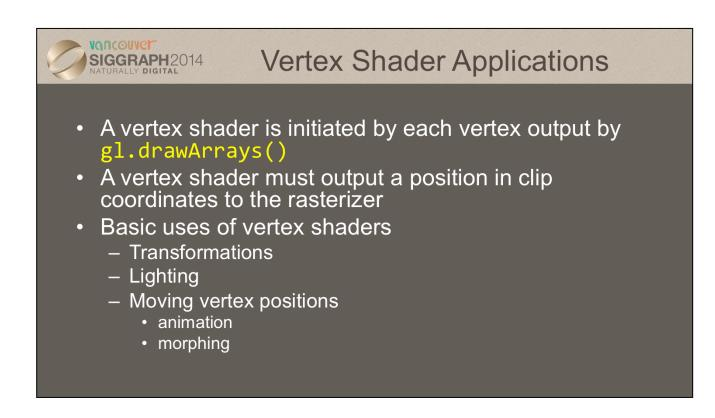
We begin delving into shader specifics by first taking a look at vertex shaders. As you've probably arrived at, vertex shaders are used to process vertices, and have the required responsibility of specifying the vertex's position in clip coordinates. This process usually involves numerous vertex transformations, which we'll discuss next. Additionally, a vertex shader may be responsible for determine additional information about a vertex for use by the rasterizer, including specifying colors.
