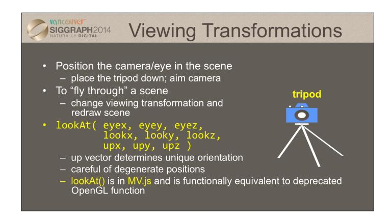
lookAt() generates a viewing matrix based on several points. lookAt() provides natrual semantics for modeling flight application, but care must be taken to avoid degenerate numerical situations, where the generated viewing matrix is undefined.
