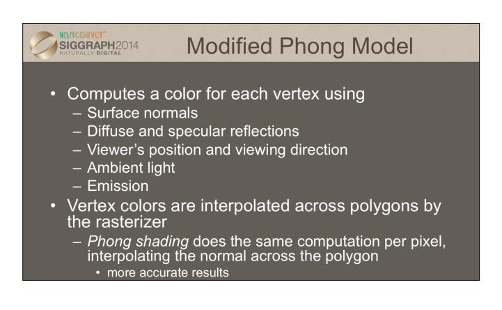
WebGL can use the shade at one vertex to shade an entire polygon (constant shading) or interpolate the shades at the vertices across the polygon (smooth shading), the default.
