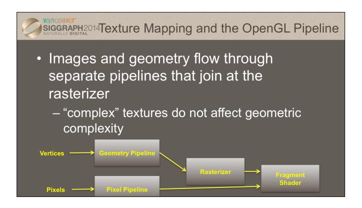
The advantage of texture mapping is that visual detail is in the image, not in the geometry. Thus, the complexity of an image does not affect the geometric pipeline (transformations, clipping) in OpenGL. Texture is added during rasterization where the geometric and pixel pipelines meet.
