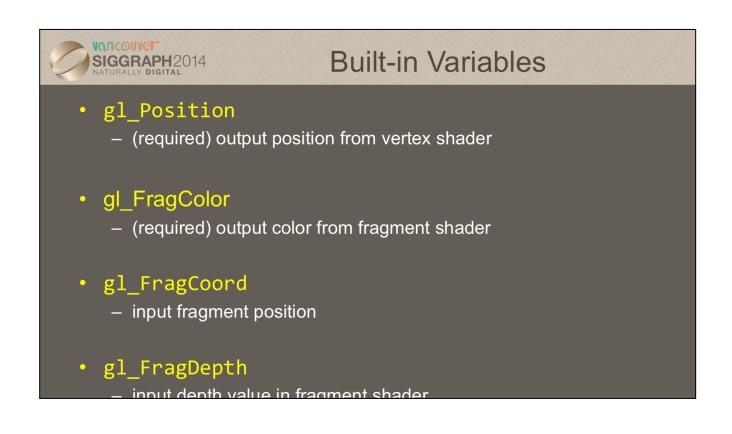
Fundamental to shader processing are a couple of built-in GLSL variable which are the terminus for operations. In particular, vertex data, which can be processed by up to four shader stages in OpenGL, are all ended by setting a positional value into the built-in variable, gl\_Position.
