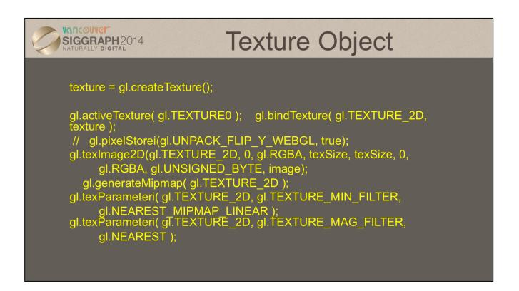
The above functions completely specify a texture object. The code creates a texture id by calling gl.createTexture(). It then binds the texture using gl.bindTexture() to open the object for use, and loading in the texture by calling gl.texImage2D(). After that, numerous sampler characteristics are set, including the texture wrap modes, and texel filtering.
