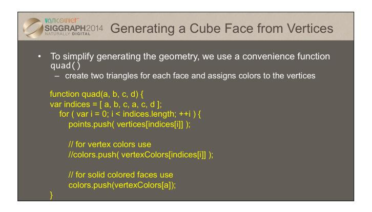
As our cube is constructed from square cube faces, we create a small function, quad(), which takes the indices into the original vertex color and position arrays, and copies the data into the VBO staging arrays. If you were to use this method (and we'll see better ways in a moment), you would need to remember to reset the Index value between setting up your VBO arrays.
