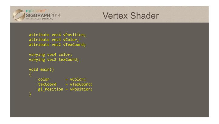
In order to apply textures to our geometry, we need to modify both the vertex shader and the pixel shader. Above, we add some simple logic to pass-thru the texture coordinates from an attribute into data for the rasterizer.
