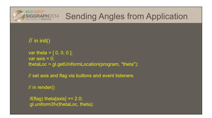
Finally, we merely need to supply the angle values into our shader through our uniform plumbing. In this case, we track each of the axes rotation angle, and store them in a vec3 that matches the angle declaration in the shader. We also keep track of the uniform's location so we can easily update its value.
