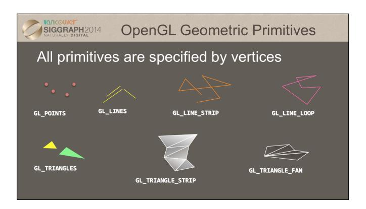
To form 3D geometric objects, you need to decompose them into geometric primitives that WebGLcan draw. WebGL (and modern desktop OpenGL) only knows how to draw three things: points, lines, and triangles, but can use collections of the same type of primitive to optimize rendering.
