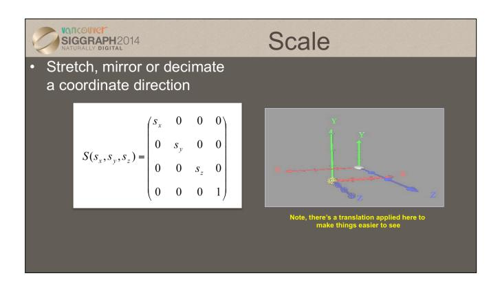
Here we show the construction of a scale matrix, which is used to change the shape of space, but not move it (or more precisely, the origin). The above illustration has a translation to show how space was modified, but a simple scale matrix will not include such a translation.
