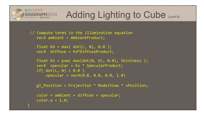
Here we complete our lighting computation. The Phong model, which this shader is based on, uses various material properties as we described before. Likewise, each light can contribute to those same properties. The combination of the material and light properties are represented as our "product" variables in this shader. The products are merely the component-wise products of the light and objects same material propreties. These values are computed in the application and passed into the shader.
