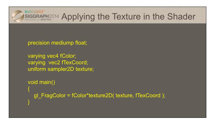
Just like vertex attributes were associated with data in the application, so too with textures. In particular, you access a texture defined in your application using a *texture sampler* in your shader. The type of the sampler needs to match the type of the associated texture. For example, you would use a sampler2D to work with a two-dimensional texture created with gl.texImage2D( GL\_TEXTURE\_2D, ... );
