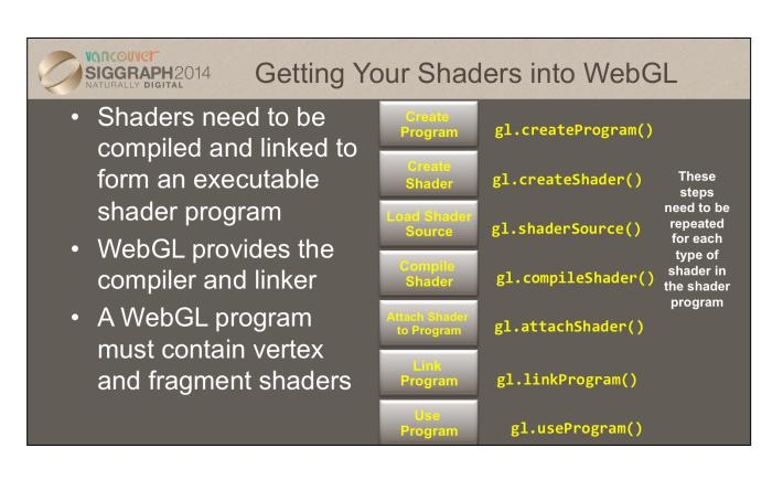
Shaders need to be compiled in order to be used in your program. As compared to C programs, the compiler and linker are implemented in the OpenGL driver, and accessible through function calls from within your program. The diagram illustrates the steps required to compile and link each type of shader into your shader program. A program must contain a vertex shader (which replaces the fixed-function vertex processing), a fragment shader (which replaces the fragment coloring stages).
