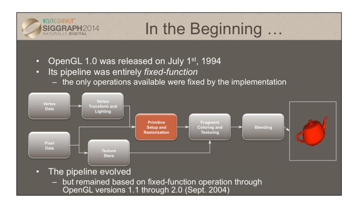
The initial version of OpenGL was announced in July of 1994. That version of OpenGL implemented what's called a *fixed-function pipeline*, which means that all of the operations that OpenGL supported were fully-defined, and an application could only modify their operation by changing a set of input values (like colors or positions). The other point of a fixed-function pipeline is that the order of operations was always the same – that is, you can't reorder the sequence operations occur.
