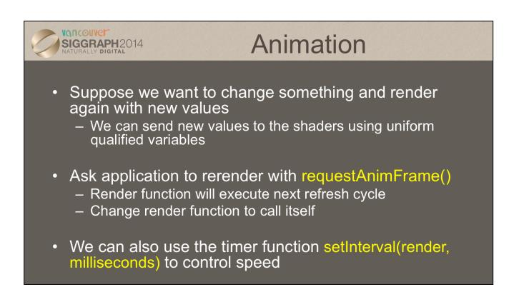
uniform qualified variables are constant for an execution of gl.drawArrays(), i.e. are constant for each instantiation of the vertex shader.
