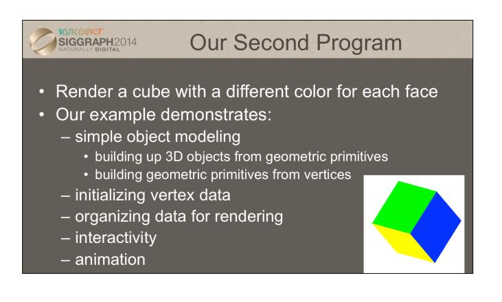
The next few slides will introduce our second example program, one which simply displays a cube with different colors at each vertex. We aim for simplicity in this example, focusing on the WebGL techniques, and not on optimal performance. This example is animated with rotation about the three coordinate axes and interactive buttons that allow the user to change the axis of rotation and start or stop the rotation.
