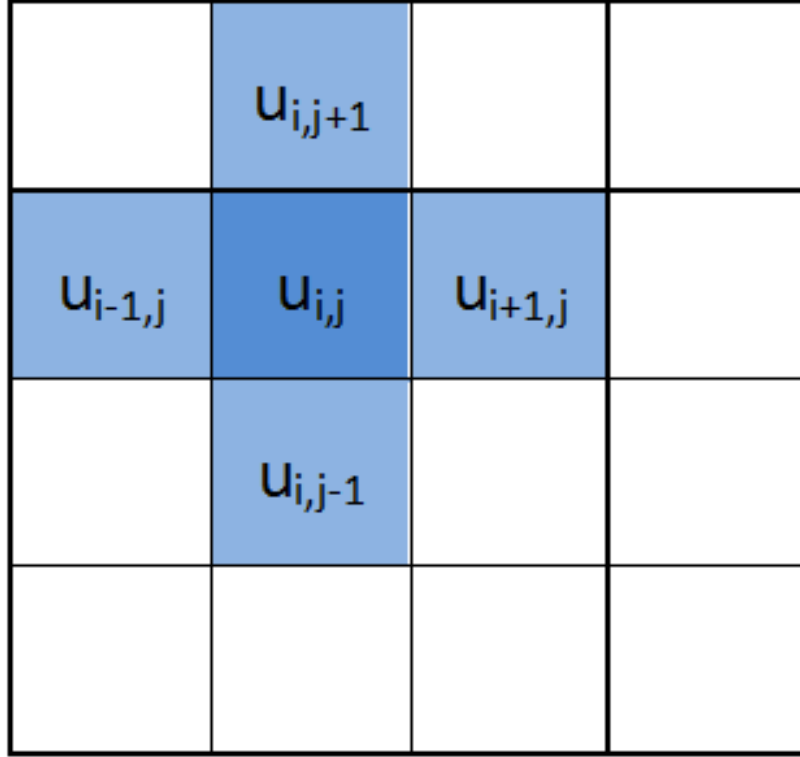
Figure 3.1: Points used for a 2D ODETLAP averaging equation
