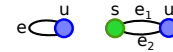
Figure 3: Loop starting point e being replaced with two artificial edges and a starting point s .
