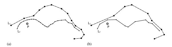
Figure 1. (a) Example of polylines  $L_1$  and  $L_2$  and a control point P. (b) Simplification of  $L_1$  and  $L_2$ . Notice that topology consistency is preserved: no intersections were created and sidedness is maintained.
