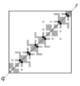
Figure 3. Geometry of the planar orientation predicate for double precision floating point arithmetic. White points represent correct outputs, gray were considered collinear and black cells points considered to be in the wrong side of the line. The diagonal line is an approximation to line (q, r).
