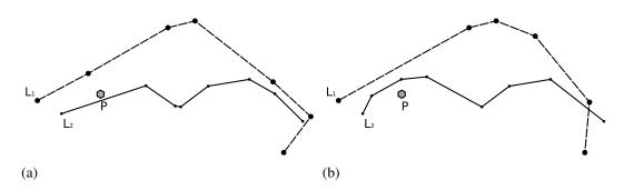
Figure 2. Inconsistent simplification output: (a) P is on the wrong side of line  $L_2$ ; (b) nonexisting nersection between lines  $L_1$  and  $L_2$  is created.
