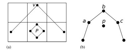
Figure 6. (a) Example where a polyline intersecting multiple cells needs to access data in a cell it does not intersect. (b) Example where the deletion of a point makes the deletion of other points infeasible .
