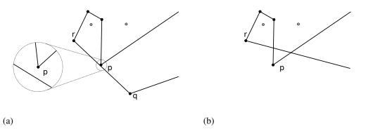
Figure 5. (a) Example input of a single line and the occurrence of a false outside. (b) Simplification with a false outside point. The removal of point q produces a self-intersecting line.
