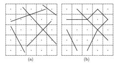
**Figure:** (a) before snap-rounding. (b) after snap-rounding. Intersections were introduced.
