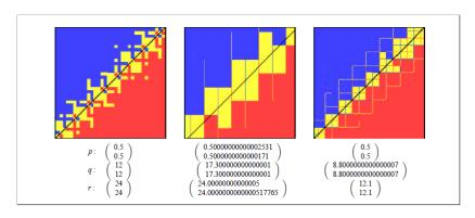
Result of the planar orientation problem using floating-point arithmetic. Source: [Kettner et al., 2008].
