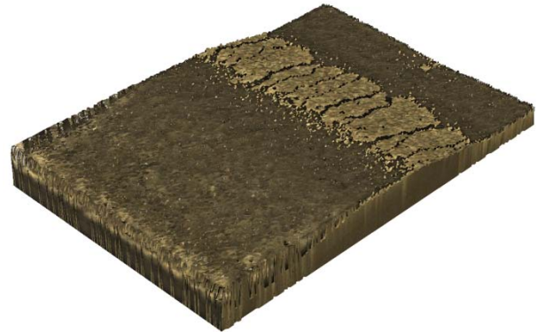
(b). Overtopping and formation of rills
