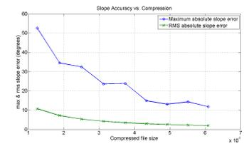
Fig. 1. Slope accuracy under lossy compression
