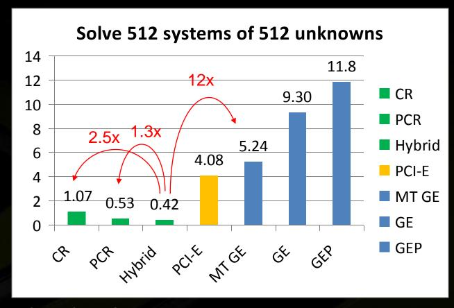
PCI-E: CPU-GPU data transfer
