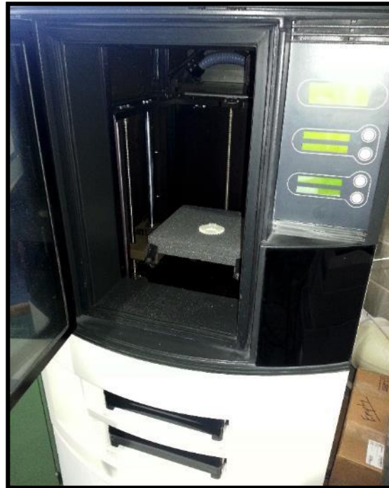
Figure 11: Stratasys Dimension Machine with printed part
