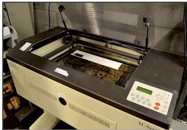
Figure 1: RPI Laser Cutting Machine showing sheet work piece (in white)
