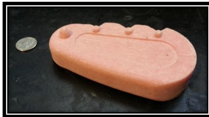
Figure 14: Z-Corp plaster printed part with post-processing (Wax Coated)
