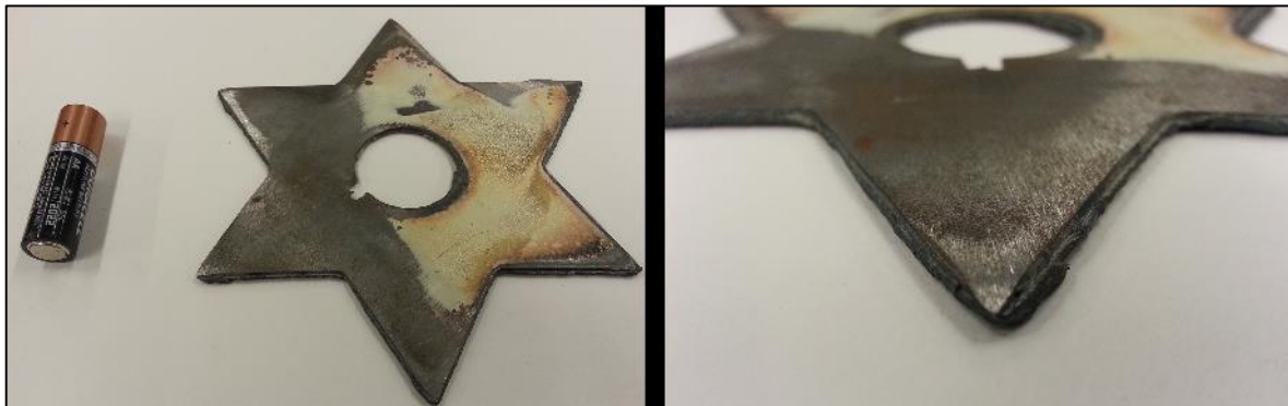
Figure 3: Plasma-cut shape (left) and close-up of edge effects after cut (right)
