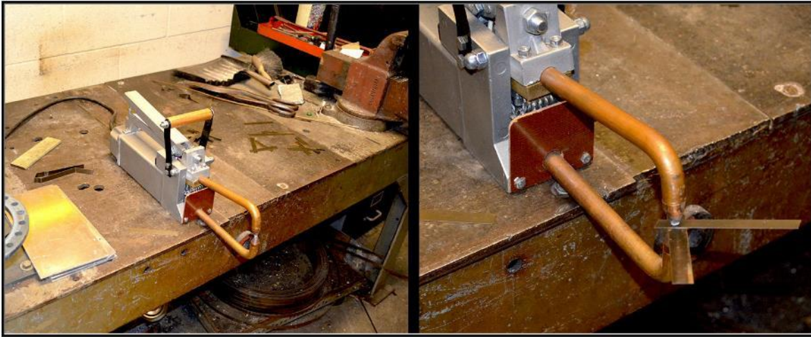
Figure 4: Spot Welding Machine (Left) and Close-Up prepared with two sheet-metal work-pieces (Right)
